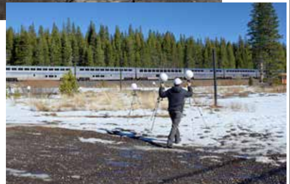
From top: Art Clark laying out his accouterments. Christopher Oudegeest laying out LIDAR equipment containers. Christopher Oudegeest with the 3d scanner set up. Christopher Oudegeest setting out small balls to mark building corners. Large balls "register" scans to put scans together. Photos by George Lamson
